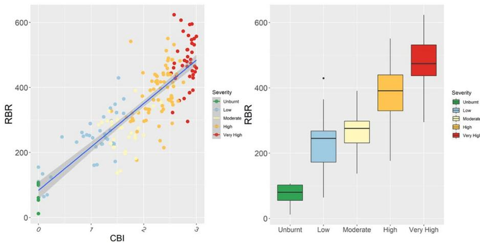
FIGURE 1. CANOPY BURN INDEX (CBI) VERSUS REMOTELY SENSED RELATIVE BURN RATION (RBR) WITH SEVERITIES IN COLOUR (A) AND BOXPLOTS OF RBR BY SEVERITY CLASS (B). A SIMPLE LINEAR REGRESSION OF THE DATA IN (A) YIELDS AN  $R^2=0.71$ . BREAKS BETWEEN CLASSES ARE LARGELY WELL RESOLVED IN BOXPLOTS EXCEPT LOW VS MODERATE.
