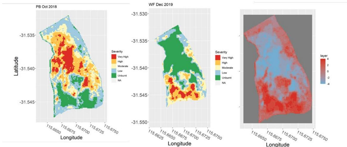
FIG 8. BURN SEVERITY IN A PRESCRIBED BURN (A; 25 OCT 2018), YANCHEP BUSHFIRE (11-12 DEC 2019), AND THE DIFFERENCE IN SEVERITY CLASSES BETWEEN THE TWO EVENTS. CLEAR INTERACTION IS APPARENT BETWEEN THE BURN AND BUSHFIRE WITH NOTABLE LOW-LOW AND MOD-MOD AREAS IN THE NE REGION OF THE AREA.
