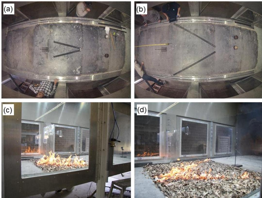
**Figure 6:** Photographs of experimental set up and experimental fires conducted in the CSIRO Pyrotron as part of the experimental program. Panel (a) shows the ignition pattern for the 800 mm, 15° inflection and zero separation case, while panel (b) shows the same for the 1500 mm, 30° inflection and 150 mm separation case. Panel (c) shows the 800 mm, 30° inflection, no wind experiment underway, while panel (d) shows the 1500 mm, 30°, 1 m s<sup>-1</sup> wind experiment underway.
