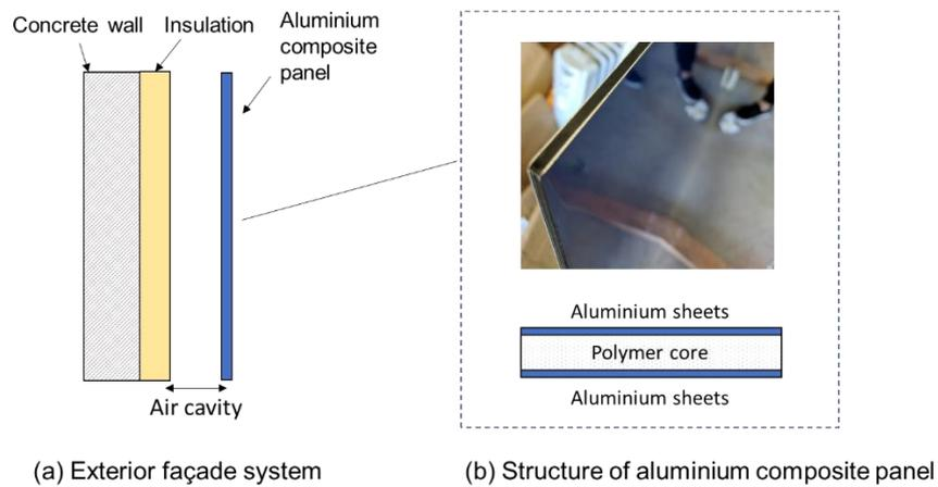
**Figure 1: Diagram of (a) components of an exterior façade system and (b) the structure of the aluminium composite panel.**
