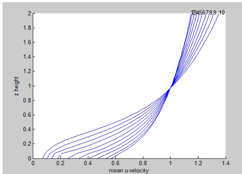
Figure 2: Mean centreline  $u$ -velocity profile over the canopy for a 1/7-power law input profile. (1) is in the canopy-free region, and (10) is at the end of the canopy. Note the velocity profile has been normalised by the velocity at the top of the canopy, and the results is preliminary.
