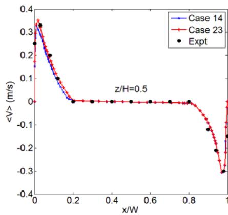
Figure 10. Computed and measured velocity profiles at the mid-height of a differentially heated cavity.
