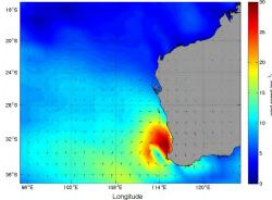
**Figure 3.** Snapshot of JRA-55 model wind speeds for cyclone Alby on 4 April 1978 used to force the hydrodynamic/surge model. Intense winds over a broad area created extreme surges along the SW Australian coastline.
