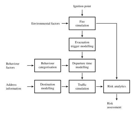
Figure 1: Modelling flow diagram
