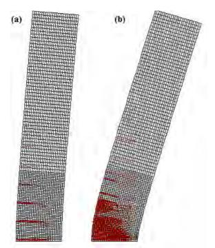
FIGURE 6 CRACKING DISTRIBUTION RESULTS FROM VECTOR2 AT ULTIMATE DISPLACEMENT WITH (a)  $\rho_{w}$ =0.70 % AND (b)  $\rho_{w}$ =0.75 %
