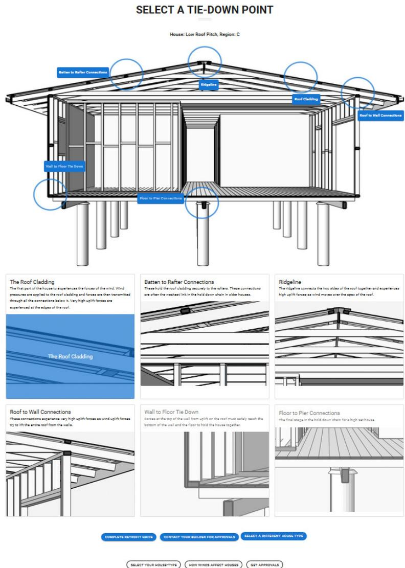
FIGURE 5 AN EXAMPLE OF THE INTERACTIVE INFOGRAPHICS FOR HIGHSET, LOW ROOF PITCH HOUSE TYPE
