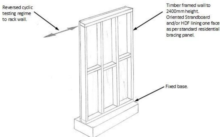
(B) MANUFACTURED SHEET WALL BRACING
