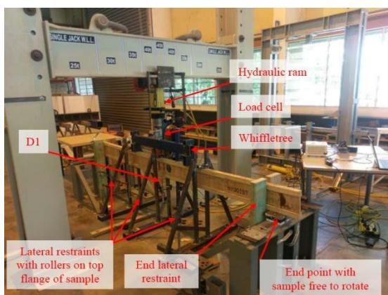
(C) ENGINEERED TIMBER JOISTS
