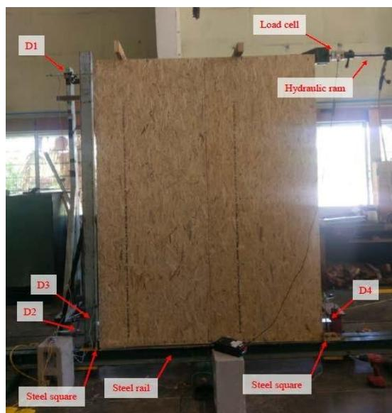
(B) MANUFACTURED SHEET WALL BRACING
