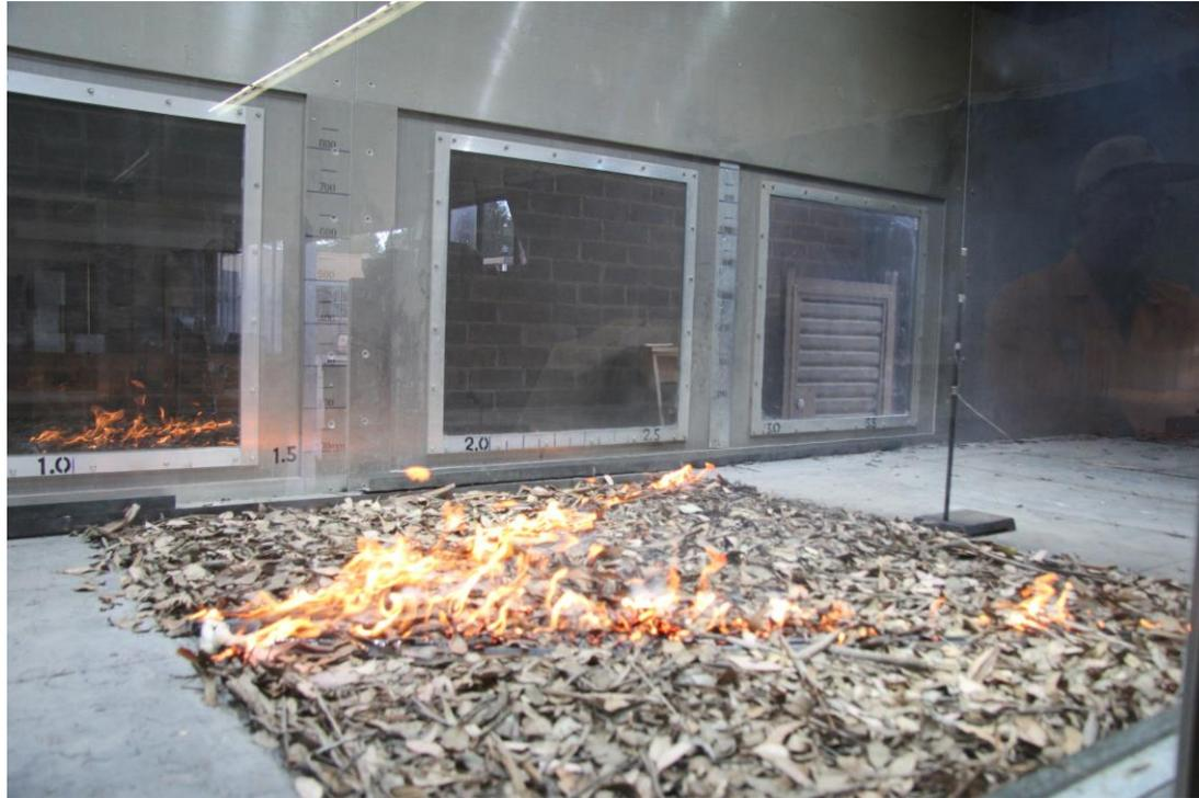
**Figure 2:** Photograph of experimental V-fire in the CSIRO Pyrotron. It shows the 800mm arms at an angle of 45° with a 1 m/s wind. Pronounced fire activity is evident in the vicinity of the point of intersection of the arms of the V.
