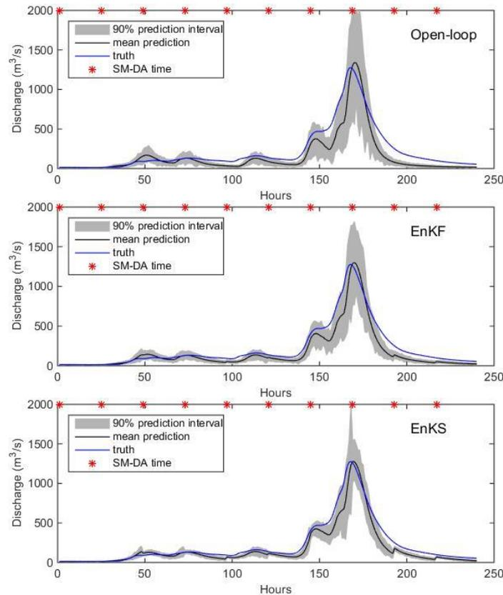
FIGURE 3 ENSEMBLE STREAMFLOW PREDICTION BEFORE AND AFTER DATA ASSIMILATION FOR AN EVENT IN 2011.
