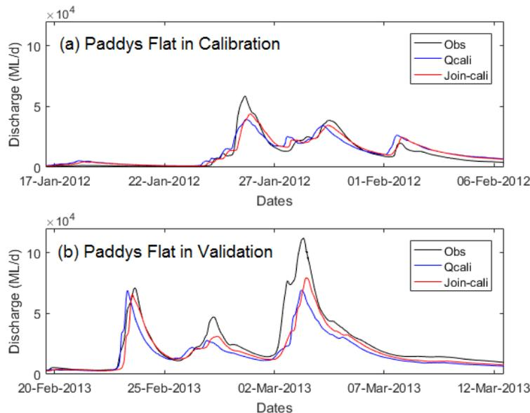
FIGURE 2 STREAMFLOW PREDICTION AT “UNGAUGED” LOCATIONS OF PADDYS FLAT SHOWING ONE FLOOD EVENT IN THE CALIBRATION PERIOD AND ANOTHER IN THE VALIDATION PERIOD.
