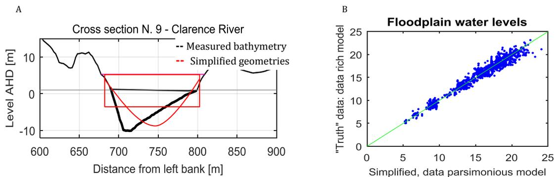
FIGURE 4A - CLARENCE RIVER, EXAMPLE OF CROSS SECTION. BLACK: FIELD DATA; MAGENTA: BANKFULL LEVEL; RED: RECTANGULAR SIMPLIFIED GEOMETRY AND EXPONENTIAL SIMPLIFIED GEOMETRY. FIGURE 4B - COMPARISON OF THE RESULTS OF DATA RICH MODEL WITH THE RESULTS OF THE SIMPLIFIED MODEL
