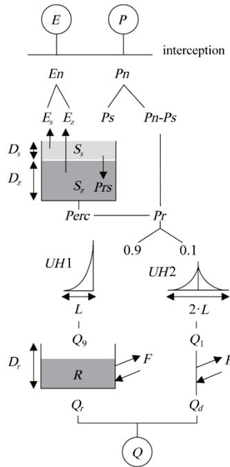
FIGURE 1 THE STRUCTURE OF THE GRKAL MODEL (FRANCOIS ET AL., 2003).
