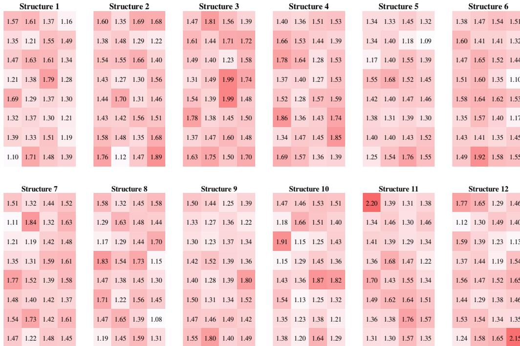
Figure 7.2 Strengths of twelve randomised connection sets [kN], based on a probability distribution determined from connection testing.
