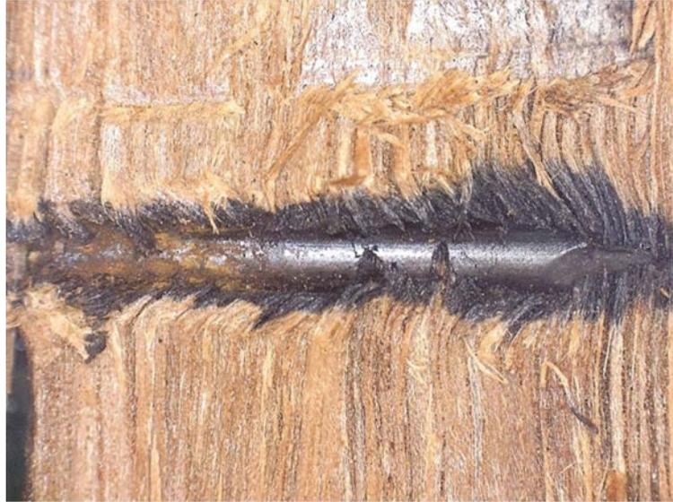
*Figure 4.5 Cross section through oven dried test specimen showing deformation of fibres due to nail penetration and dark coloured corrosion bi-product.*
