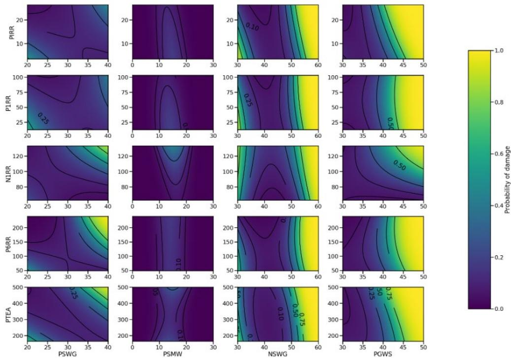
**Figure 8: Quadratic discriminant analysis (QDA) of damage arising due to combination of rainfall and wind hazards. The colours represent the probability of a building being damaged in an event with the prescribed wind and rainfall hazard levels. See Table 2 for definitions of hazard parameters. "Damaged" is defined as EICU damage ratings in the categories moderate, extensive or complete. Contour intervals are 0.25.**
