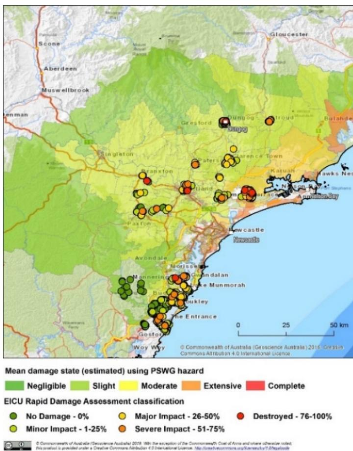
Figure 10: Rapid Damage Assessment (RDA) data from the Emergency Information Coordination Unit (EICU) overlaid on the predicted mean damage state based on BARRA-SY using the point maximum surface wind gust (PSWG) as the wind hazard for the 20-22 April 2015 Dungog ECL.
