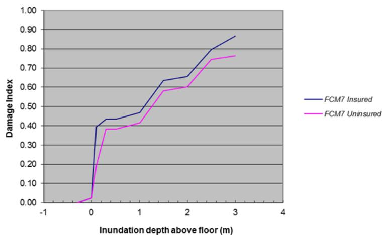
Figure 4: Analytical vulnerability function for a single storey brick veneer, slab-on-grade house exposed to riverine flood hazard (Wehner et al. 2017).
