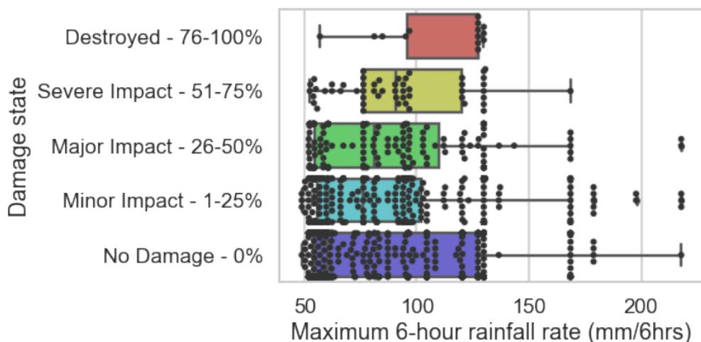
Figure 7: Fragility data from 2072 EICU damage assessments for the 20-22 April 2015 ECL storm plotted against maximum 6-hour rainfall rate (P6RR) modelled by the BARRA-SY Reanalysis.
