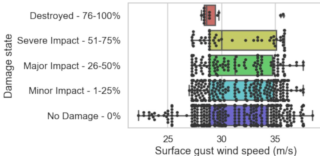
Figure 6: Fragility data from 2072 EICU damage assessments for the 20-22 April 2015 ECL storm plotted against the event maximum surface gust wind speed (PSWG) simulated by the BARRA-SY Reanalysis.
