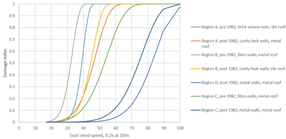
Figure 3: Heuristic vulnerability functions for a range of WA house types exposed to severe wind hazard (Boughton, 2018).
