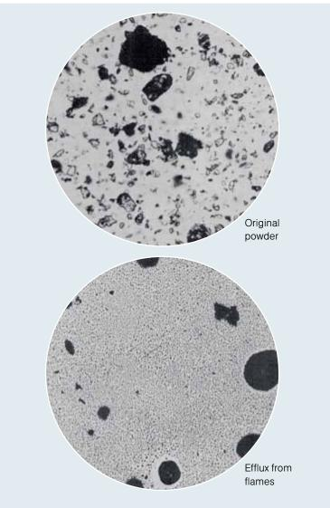
Figure 1 The effect of flames on Monnex dry chemical powder
