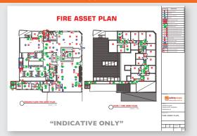
A plan that display's all the existing fire protection equipment and devices (Smoke Alarms, Fire Extinguishers, Emergency Lighting, Exit Signs, Fire Blankets, Fire Hose Reels, Manual Call Points, etc.)
