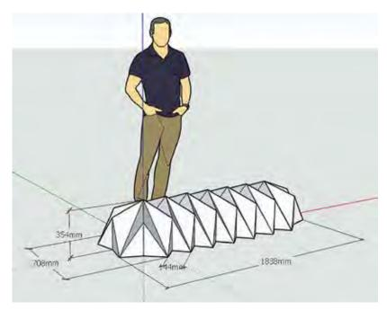
**FIGURE 3**. 3D representation of the origami fire shelter.
