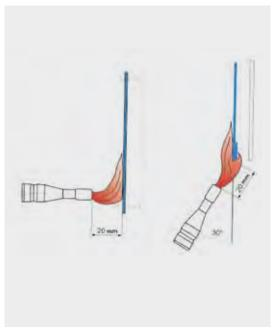
**FIGURE 4**. Procedure A (left) and procedure B (right) to ISO 15025: 2016.
