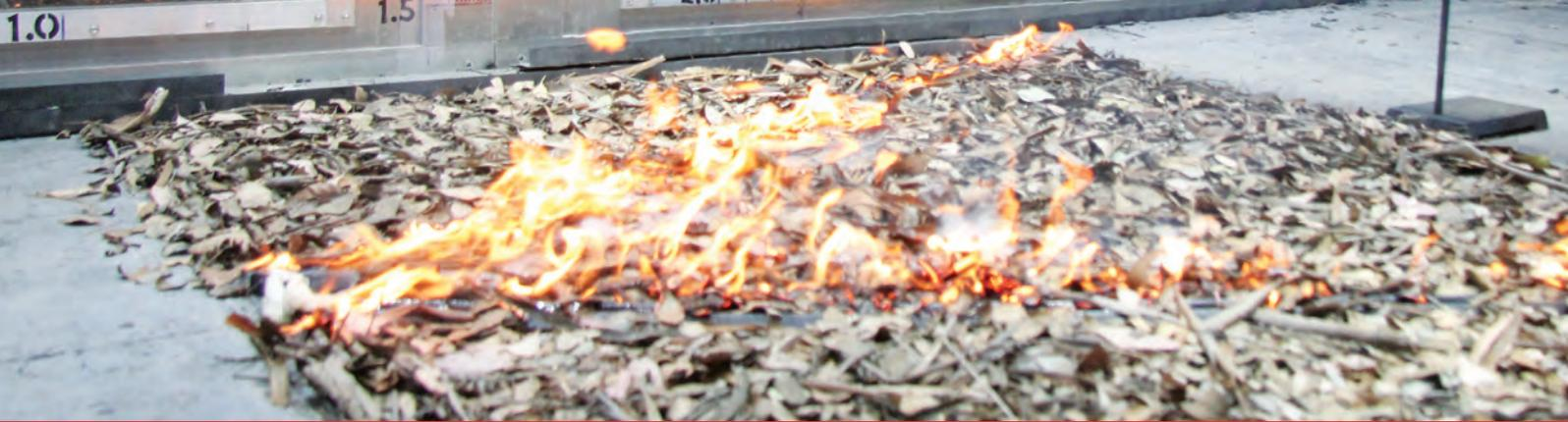
An experimental separated v-shaped fire conducted in the CSIRO Pyrotron.
