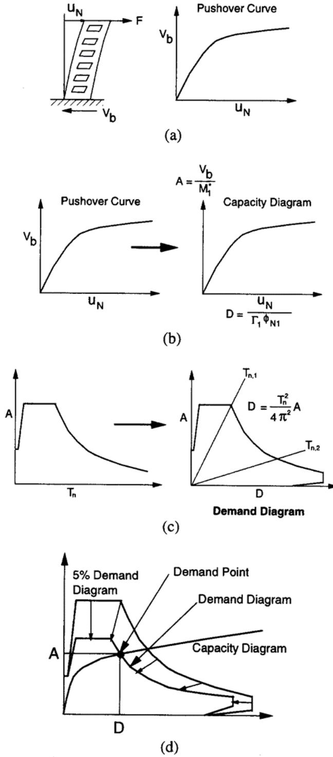
FIGURE 17 CAPACITY SPECTRUM METHOD (CHOPRA AND GOEL, 1999)
