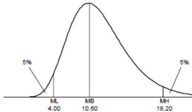
FIGURE 9 EXAMPLE OF A LOGNORMAL DISTRIBUTION OF THE ESTIMATED DAMAGE FACTOR FOR A GIVEN INTENSITY AND CLASS OF BUILDING (MCCORMACK AND RAD, 1997)
