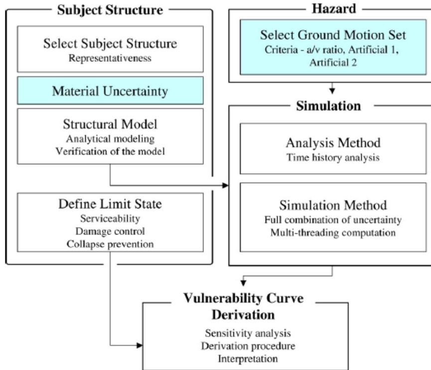
FIGURE 13 TYPICAL FLOW CHART FOR CONSTRUCTION OF ANALYTICAL VULNERABILITY CURVES (KWON AND ELNASHAI, 2006)
