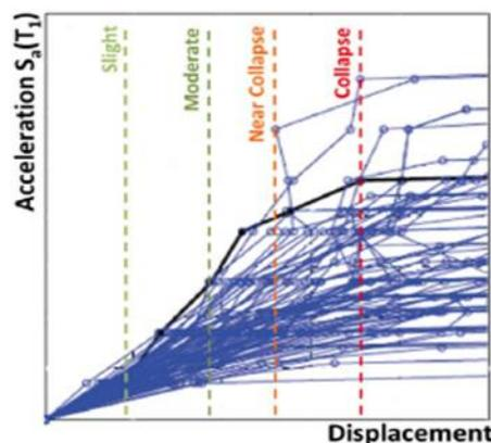
FIGURE 15 EXAMPLE PLOT OF INCREMENTAL DYNAMIC ANALYSIS CURVES (D'AYALA ET AL., 2014)
