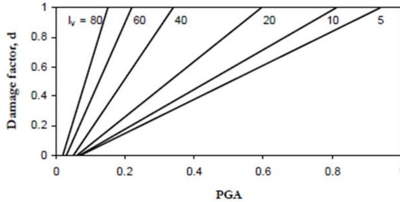
FIGURE 10 VULNERABILITY FUNCTIONS TO RELATE DAMAGE FACTOR (D) AND PEAK GROUND ACCELERATION PGA FOR DIFFERENT VALUES OF VULNERABILITY INDEX ( $I_v$ ) (GUAGENTI AND PETRINI, 1989)
