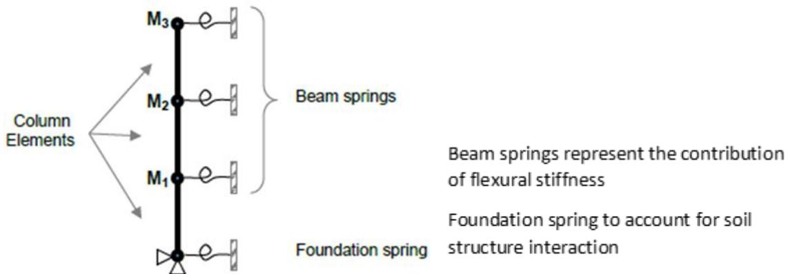
FIGURE 16 2D LUMPED MASS MDOF MODEL (D'AYALA ET AL., 2014)
