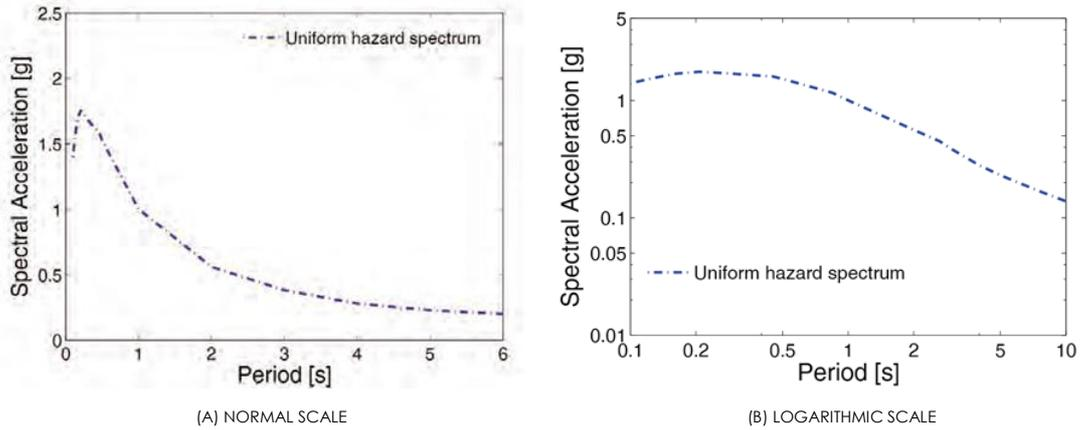
FIGURE 20 UNIFORM HAZARD SPECTRA (NEHRP, 2011)
