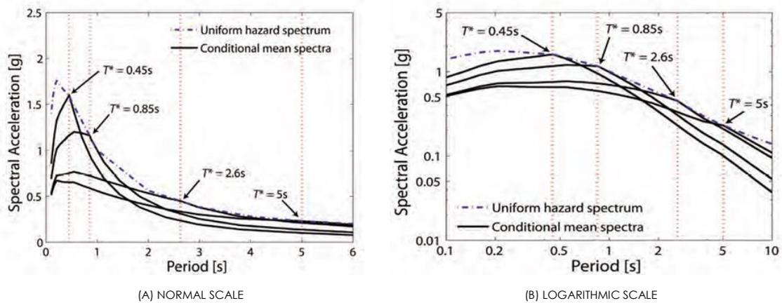
FIGURE 21 CONDITIONAL MEAN SPECTRA ANCHORED AT 0.45 SEC, 0.85 SEC, 2.6 SEC, AND 5 SEC (NEHRP, 2011)
