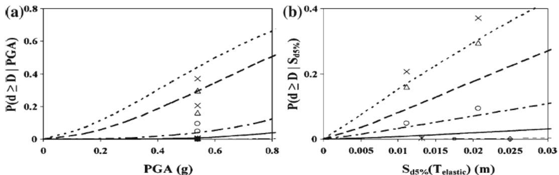
FIGURE 3 VULNERABILITY FUNCTIONS BASED ON PGA AND SD(TELASTIC) (ROSSETTO AND ELNASHAI, 2003)
