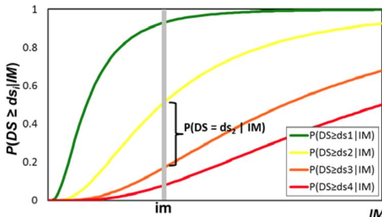
(A) FRAGILITY CURVES CORRESPONDING TO N=4 DAMAGE STATES
