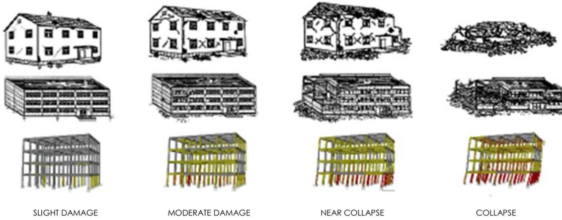
FIGURE 7 DEFINITION OF DIFFERENT DAMAGE STATES (D'AYALA ET AL., 2014)
