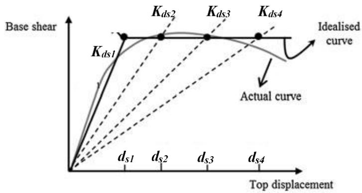
FIGURE 8 CAPACITY CURVE AND DAMAGE LIMIT STATES
