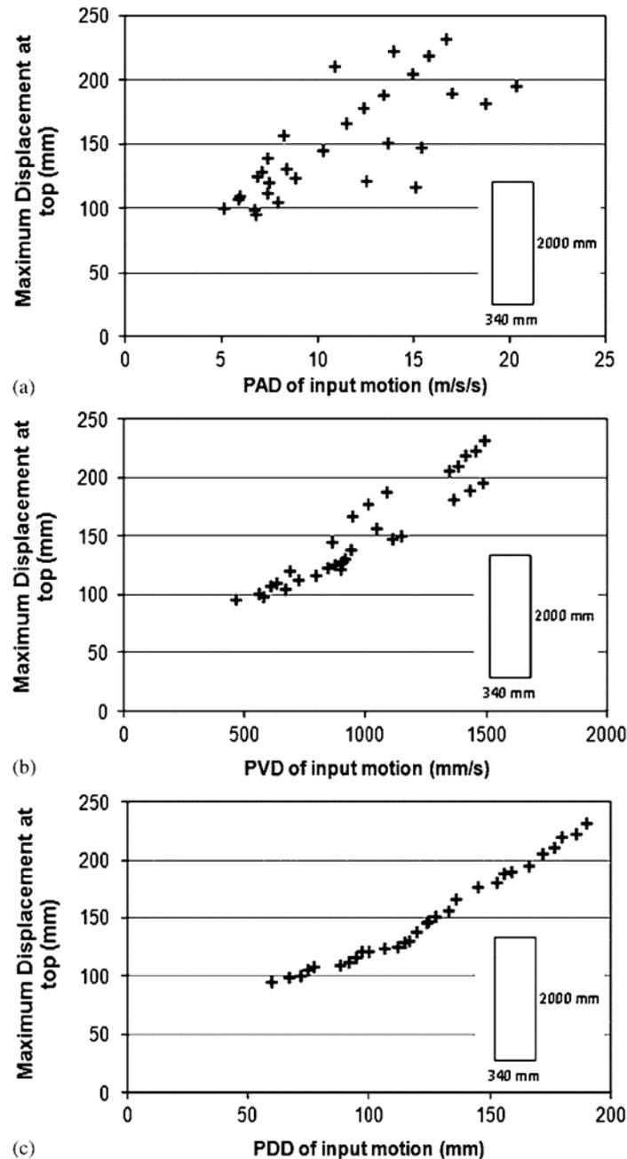
FIGURE 5 CORRELATION OF THE MAXIMUM SPECTRAL ACCELERATION (PAD), MAXIMUM SPECTRAL VELOCITY (PVD) AND MAXIMUM SPECTRAL DISPLACEMENT (PDD) WITH THE MAXIMUM DISPLACEMENT AT THE TOP OF RIGID OBJECTS (KAFLE ET AL., 2011)
