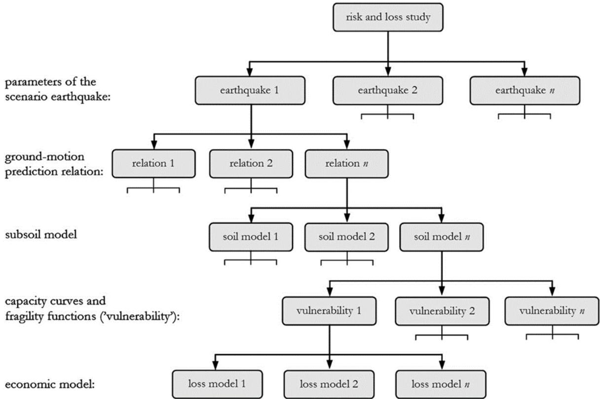
FIGURE 2 PRINCIPLE OF THE LOGIC TREE STRUCTURE IN SELENA (MOLINA ET AL., 2010)
