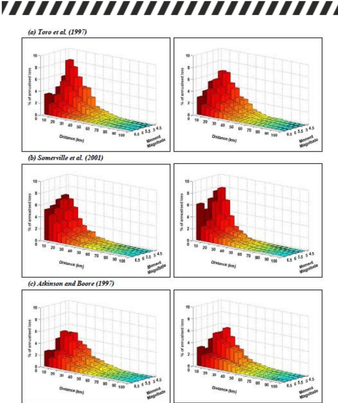
FIGURE 1 DISAGGREGATED ANNUALISED LOSS ESTIMATES IN NEWCASTLE BASED ON DIFFERENT GROUND MOTION PREDICTION MODELS (PATCHETT ET AL., 2005)
