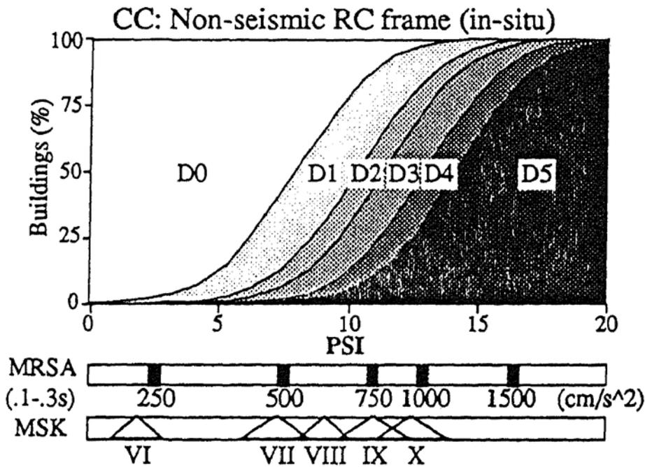
FIGURE 11 VULNERABILITY FUNCTION FOR RC FRAME BASED ON MRSA AND PSI (SPENCE ET AL., 1992)
