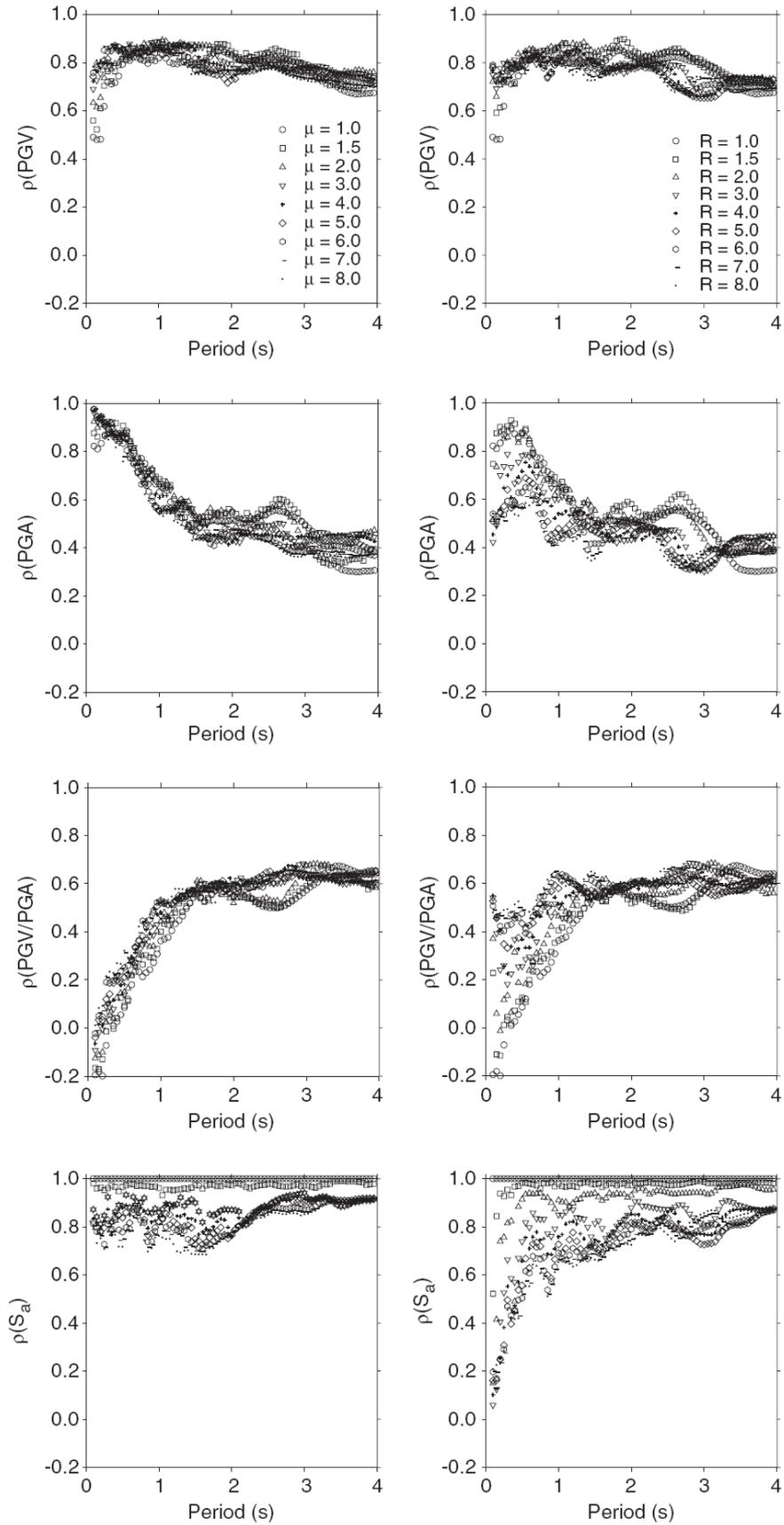
FIGURE 4 CORRELATION OF PGV, PGA, PGV/PGA AND SA WITH SDOF DISPLACEMENT DEMANDS (AKKAR AND ÖZEN, 2005)
