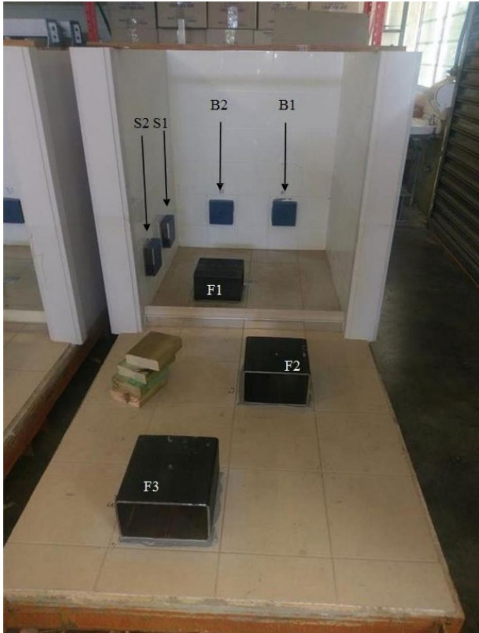
FIGURE 8: LOCATION OF TILES TO BE TESTED AND ANHOR POINTS BONDED ON TILES
