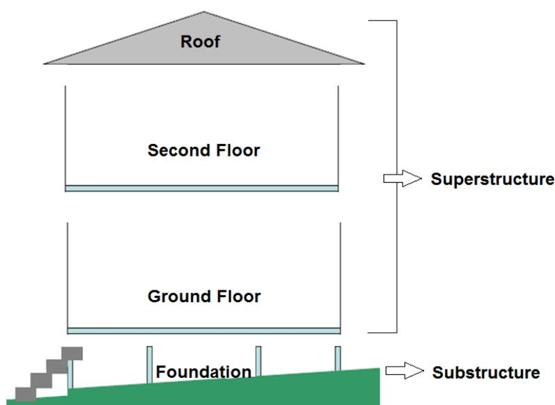
Figure 5.1 Building structure divided into main components
