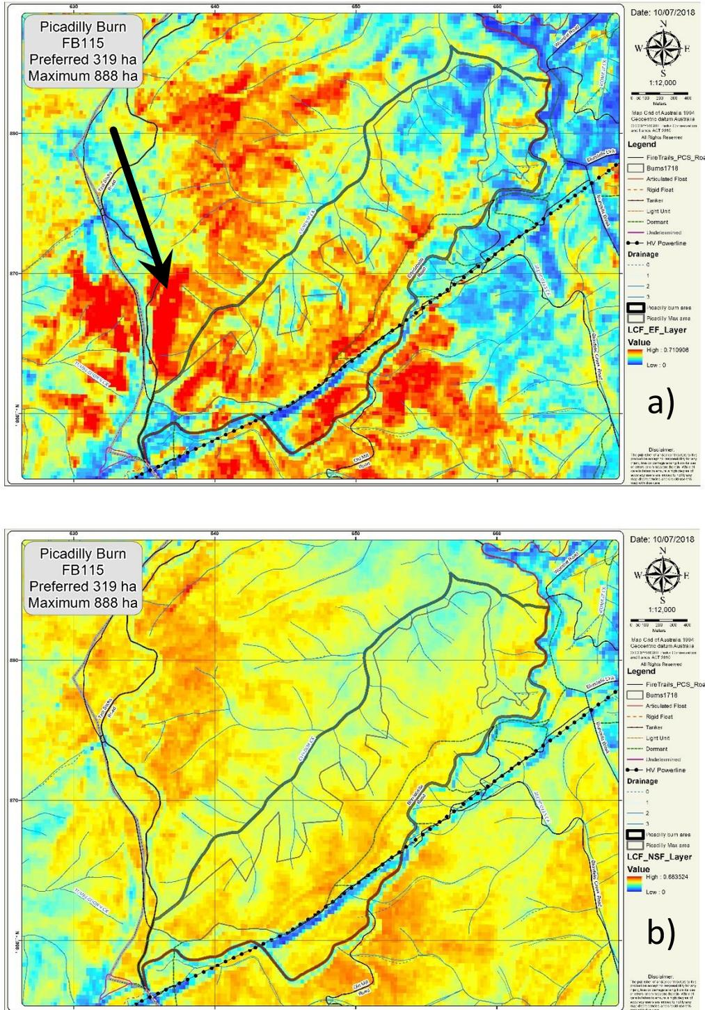
Figure 5. Experimental LiDAR-derived fuel maps for the Piccadilly burn: a = elevated fuel; b = near-surface fuel. The distribution of fuel varied considerably across the fire ground, particularly the elevated fuel. Note the dense patch of elevated fuels adjacent to the soft containment line on the western end; indicated by arrow.
