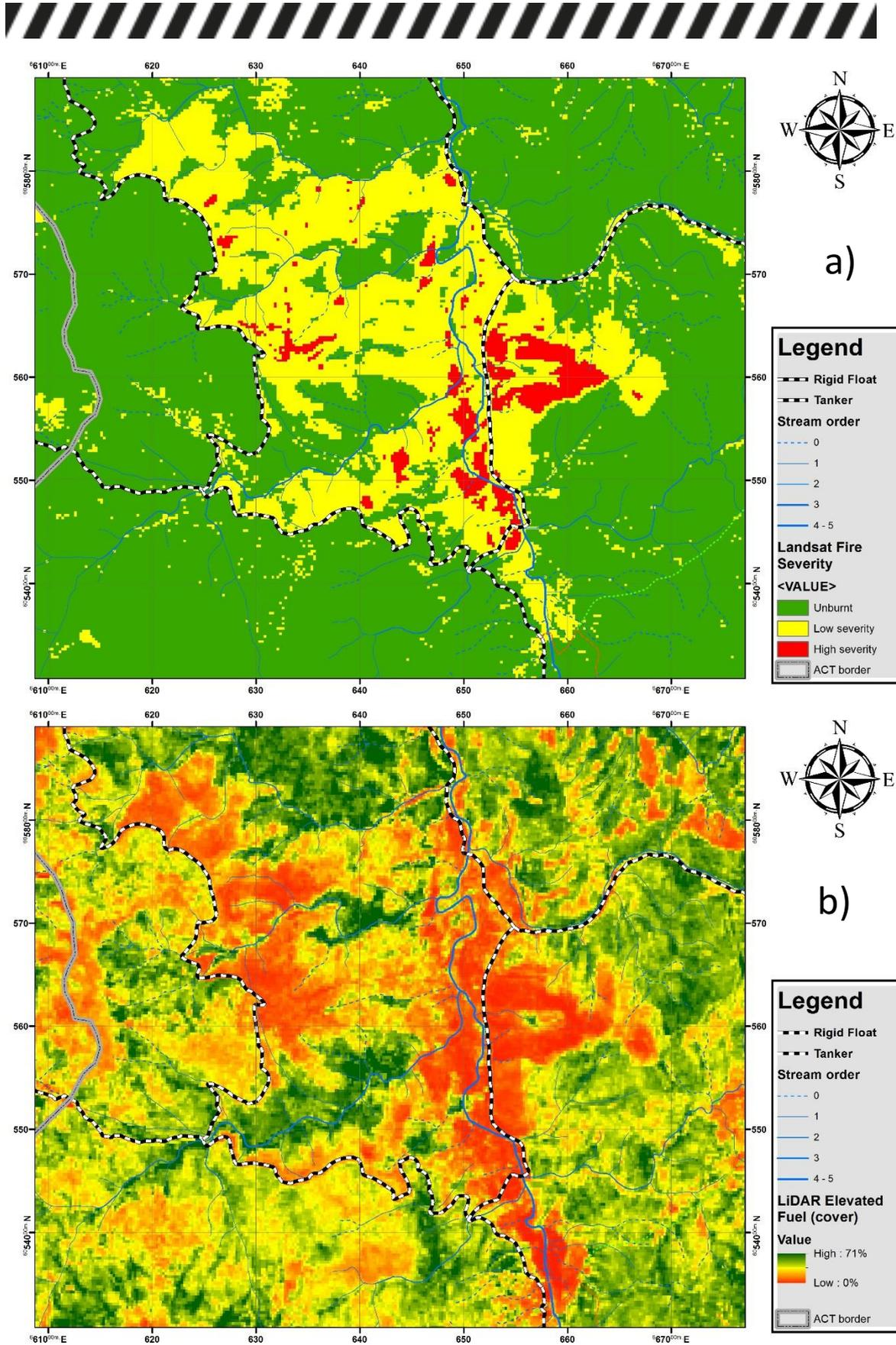
Figure 4. Comparison of the fire severity analysis (a) and LiDAR-derived elevated fuel map (b) showed good agreement.
