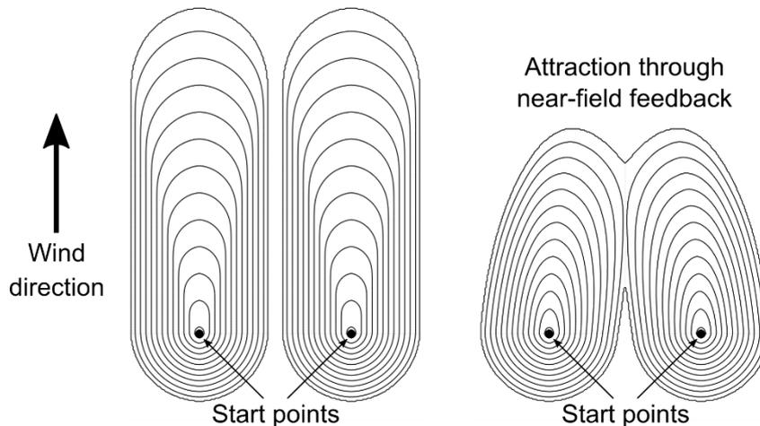
FIGURE 1 – ISOCHRONES FROM TWO FIRES SIDE-BY-SIDE WITHOUT NEAR-FIELD COUPLING (LEFT) AND WITH NEAR-FIELD COUPLING (RIGHT). THE NEAR-FIELD COUPLING THE TWO FIRES TO ATTRACT, AS IS OBSERVED IN EXPERIMENTS.
