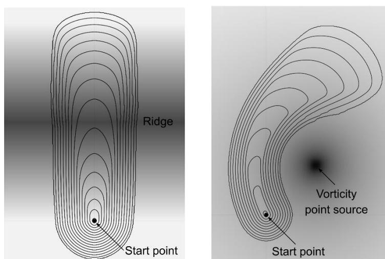
**FIGURE 3** – INCORPORATION OF TERRAIN INTO THE NEAR-FIELD MODEL AS A SOURCE TERM FOR THE SCALAR POTENTIAL (LEFT). EXAMPLE OF FIRE PROPAGATION IN THE PRESENCE OF A VORTICITY POINT SOURCE (RIGHT).
