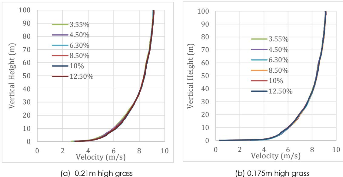
FIGURE 2 – VELOCITY PROFILES PRIOR TO THE IGNITION LOCATION FOR VARIOUS SIMULATIONS WERE RUN FOR DIFFERENT MC (FROM 3.55% TO 12.5%)
