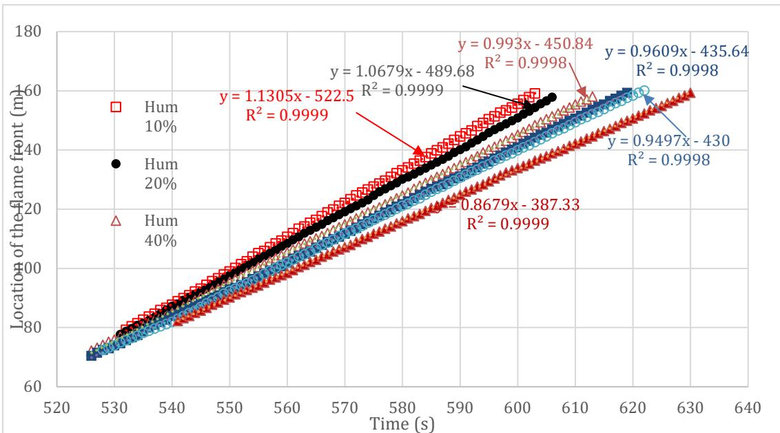
FIGURE 5 – FIREFRONT LOCATIONS VS TIME FOR CASES WITH GRASS HEIGHT OF 0.175M
