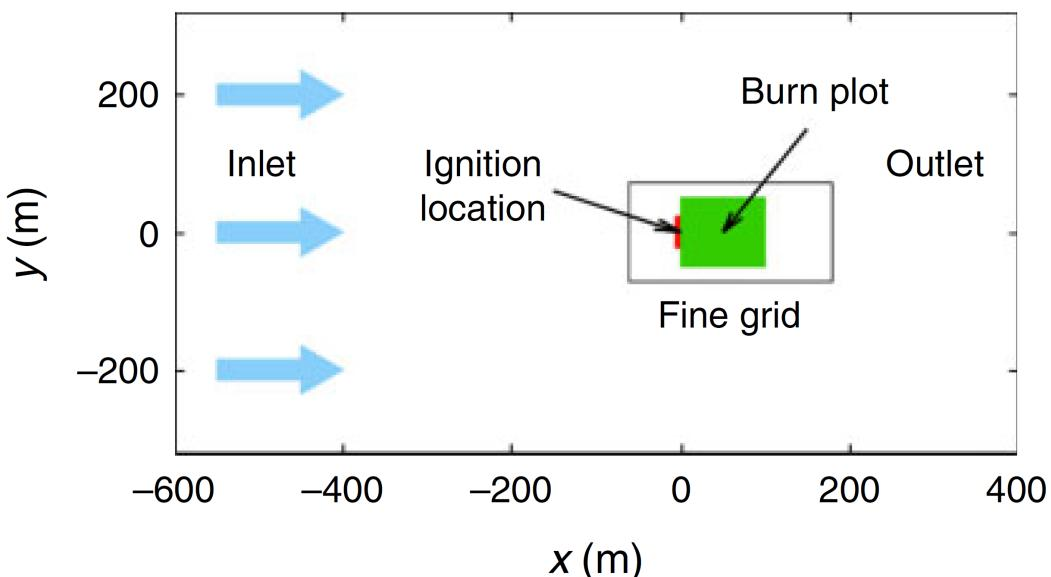
FIGURE 1 – SIMULATION DOMAIN PLAN VIEW (TAKEN FROM SUTHERLAND ET AL. [4]). THE RECTANGLE REPRESENTS AREA WITH FINE RESOLUTION OF 0.25M X 0.25M X 0.25M GRID UP TO 6M HEIGHT FROM THE GROUND.
