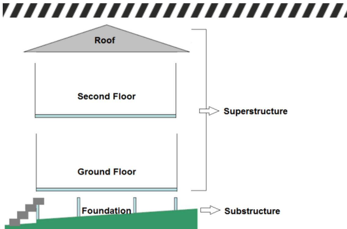
FIGURE 1: BUILDING STRUCTURE DIVIDED INTO MAIN COMPONENTS (MAQSOOD ET AL. 2015A)
