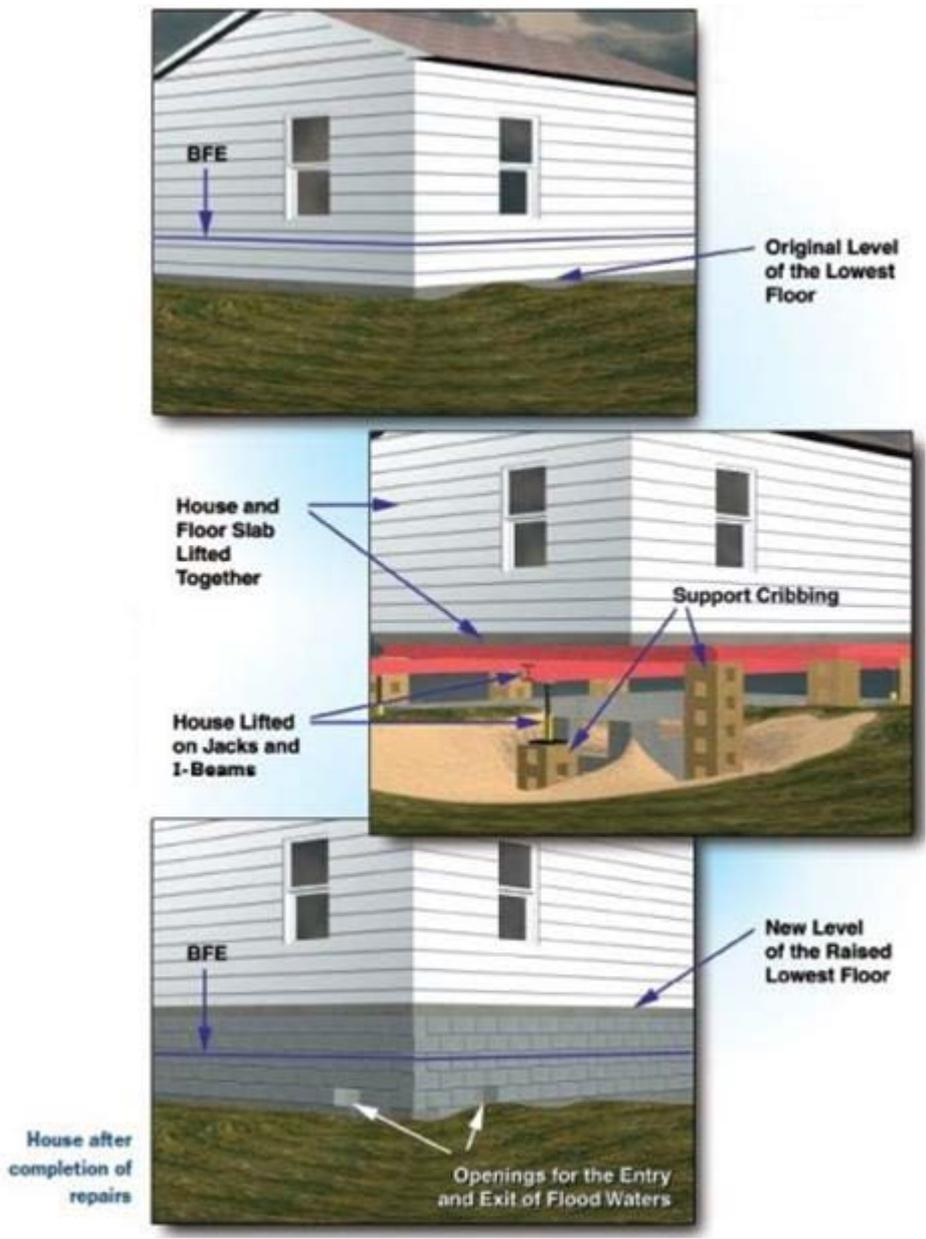
FIGURE 2: TECHNIQUES FOR ELEVATION (FEMA, 2000)
