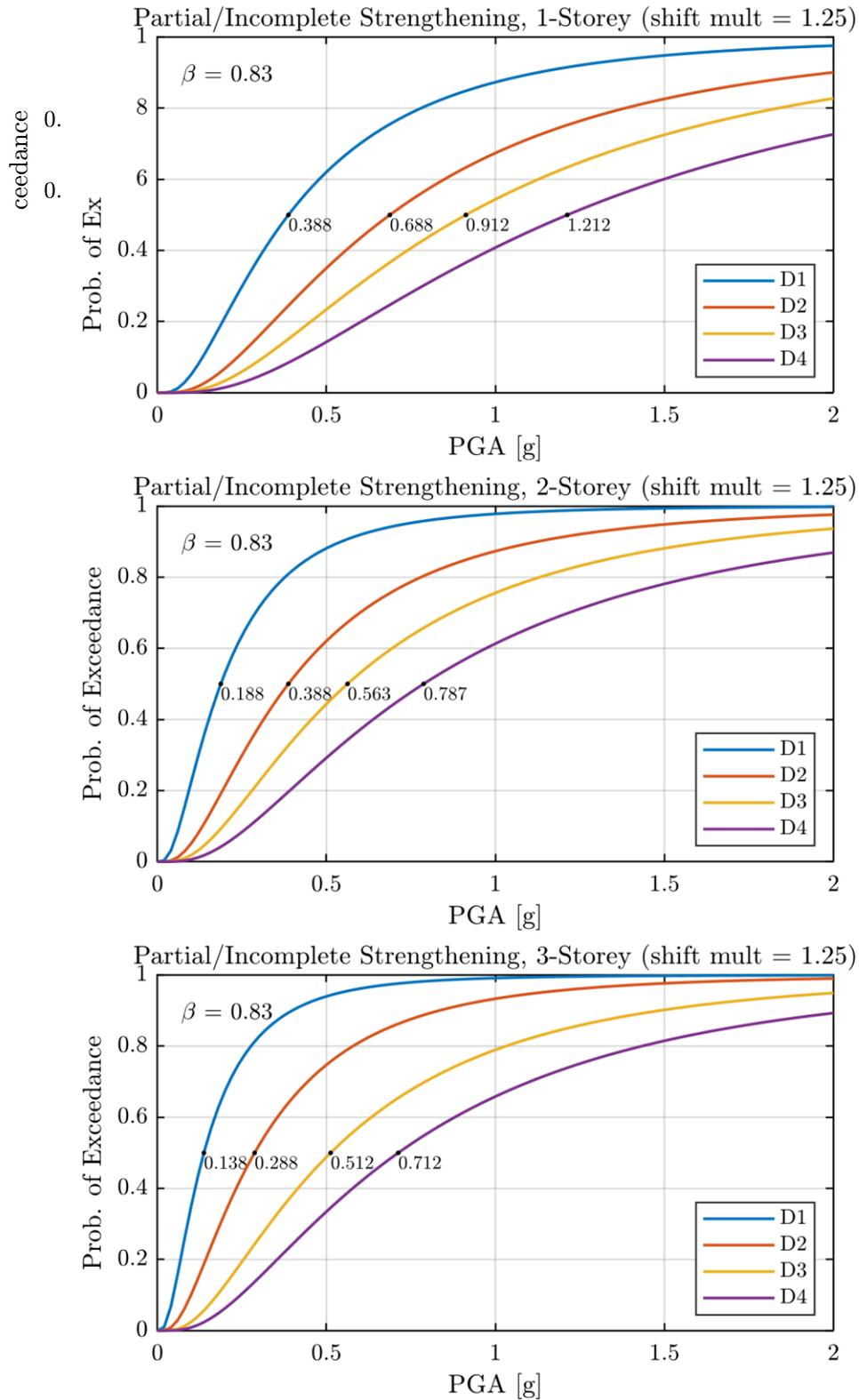
Figure 2: Fragility curves for buildings with partial/incomplete strengthening: 1, 2 and 3 storey.
