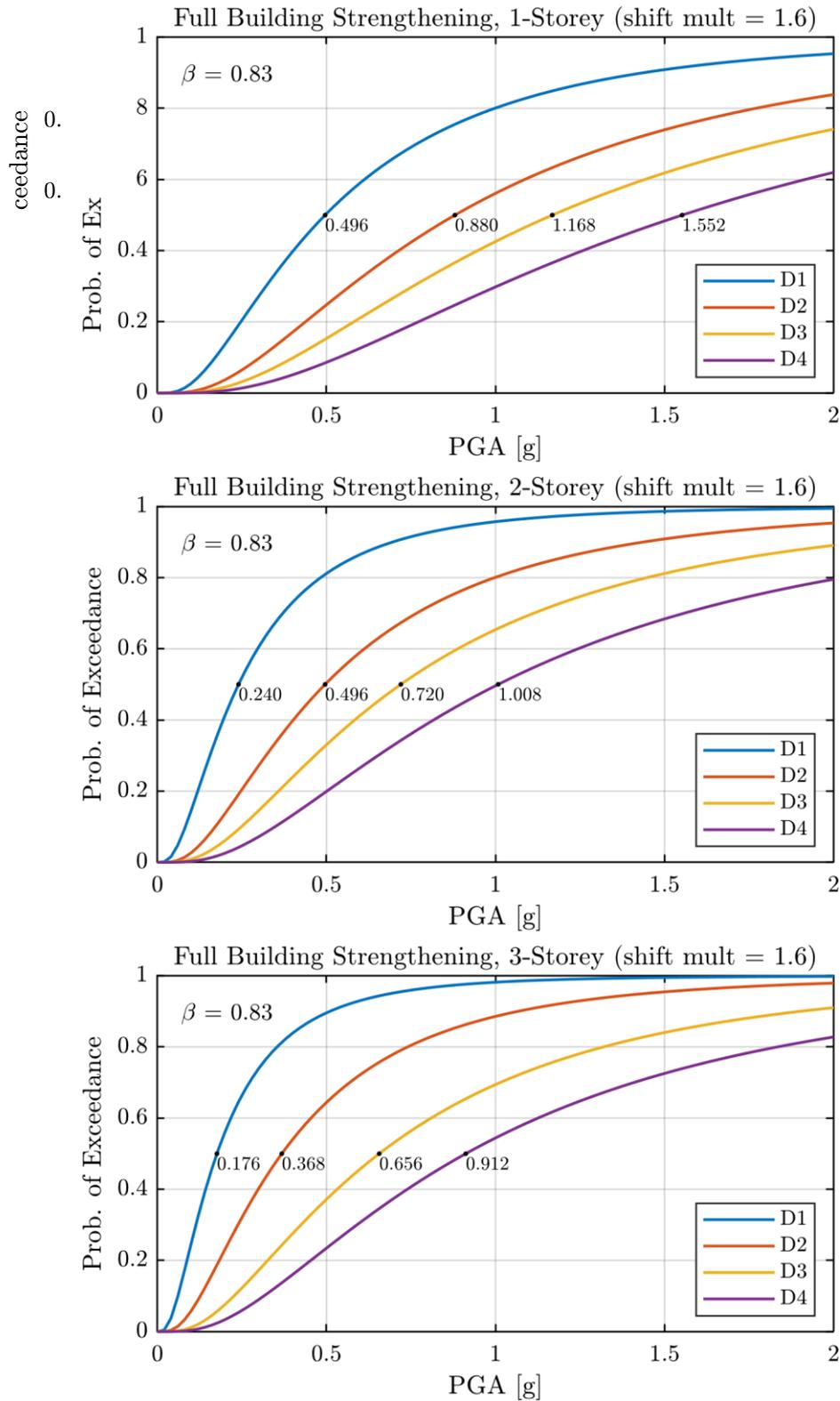
Figure 3: Fragility curves for buildings with full building strengthening: 1, 2 and 3 storey.
