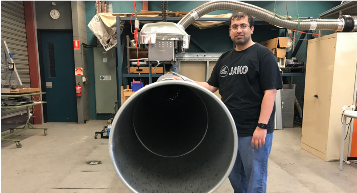
Rahul Wadhvani in the lab with the fire dragon firebrand simulator.
