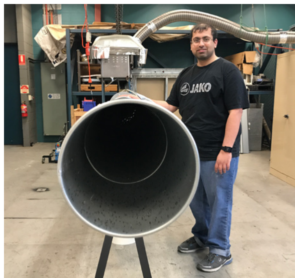
Rahul Wadhvani (Victoria University) in the lab with the fire dragon machine that measures ember spread.
