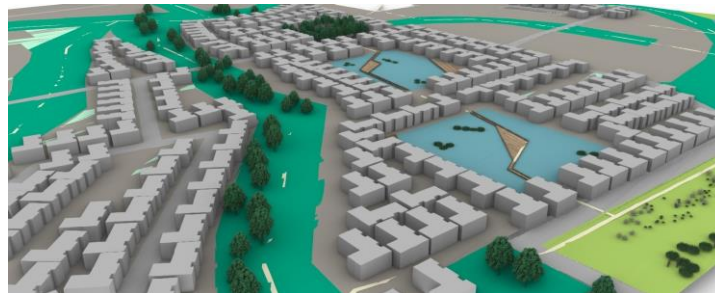
Image: A design exploration of a NATL (treated greywater located within urban development acting as landscape cooling, possibly reducing the spread of fire and as a source of local water for fire-fighting (Anna Durkin, 2023).
