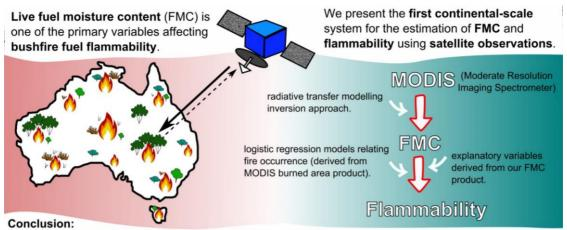
The overall accuracy of the **FMC** algorithm was **moderate** with higher uncertainties at higher FMC values. **FMC** was converted to **Flammability** using three separate logistic models for **grasslands**, **shrublands** and **forest**. These models offer the possibility of **accurately predicting fires one week** before the beginning of the event.
