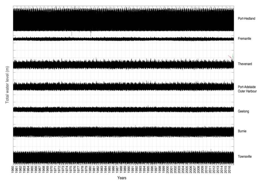
FIGURE 5. SIMULATED TOTAL WATER LEVELS, STARTING IN FREMANTLE, WA AND MOVING ANTICLOCKWISE AROUND THE COAST. DATA PLOTTED WITH ARBITRARY OFFSET AND TICK MARKS AT 1 M INTERVALS ON THE Y-AXIS. EVENTS AT THEVENARD. SA INDICATED WITH RED/GREEN ARROWS.
