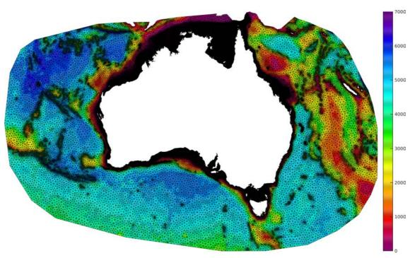
FIGURE 2. SCHISM UNSTRUCTURED MODEL MESH WITH COLOURS INDICATING DEPTH IN METRES.
