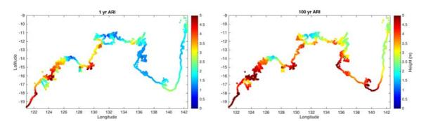
FIGURE 12. ESTIMATES OF 1YEAR AND 100 YEAR TOTAL SEA LEVEL ARI FOR NORTHERN AUSTRALIA DERIVED FROM THE NUMERICAL MODEL (COLOURED DOTS) AND TIDE GAUGE OBSERVATIONS (BLACK BORDERED CIRCLES).
