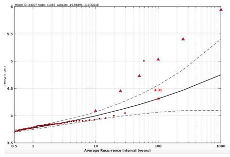
FIGURE 22. EXAMPLE PLOT OF ARI CURVE AVAILABLE FOR EACH COASTAL DATA POINT ON UWA/BNHCRC EXTREME SEA LEVEL WEBSITE WITH EXPLANATION OF CONTENTS.
