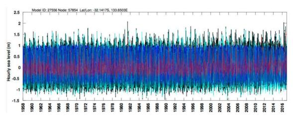
FIGURE 27. EXAMPLE TIME SERIES HOURLY DATA AVAILABLE FOR DOWNLOAD AT EACH COASTAL DATA POINT FROM THE UWA/BNHCRC WEBSITE. HERE, TIDAL ANALYSIS HAS BEEN PERFORMED ON THE DATA AND PLOTTED ARE: MSL ADJUSTED TOTAL WATER LEVELS (BLACK), PREDICTED TIDES (DARK BLUE), AND NON-TIDAL RESIDUALS (RED), AND RAW MODEL DATA (CYAN).
