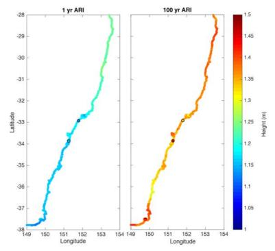
FIGURE 17. ESTIMATES OF 1YEAR AND 100 YEAR TOTAL SEA LEVEL ARI FOR NSW DERIVED FROM THE NUMERICAL MODEL (COLOURED DOTS) AND TIDE GAUGE OBSERVATIONS (BLACK BORDERED CIRCLES).
