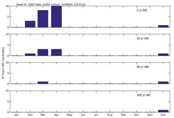
FIGURE 24. HISTOGRAM AVAILABLE ON THE UWA/BNHCRC WEBSITE INDICATING WHEN ARI LEVELS WERE EXCEEDED BETWEEN 1958-2016 IN THE SCHISM NUMERICAL MODEL SEALEVEL HINDCAST.
