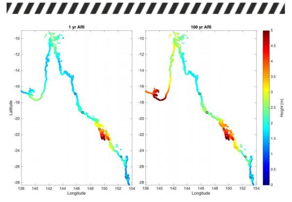
FIGURE 18. ESTIMATES OF 1 YEAR AND 100 YEAR TOTAL SEA LEVEL ARI FOR QUEENSLAND DERIVED FROM THE NUMERICAL MODEL (COLOURED DOTS) AND TIDE GAUGE OBSERVATIONS (BLACK BORDERED CIRCLES).
