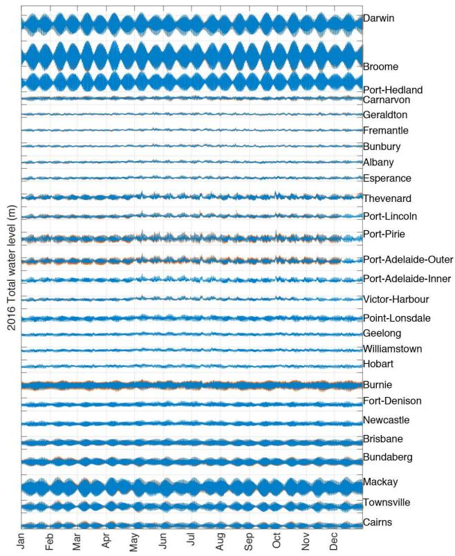
FIGURE 8. PREDICTED (BLUE) AND OBSERVED (ORANGE) TOTAL SEA LEVELS FOR 2016 PLOTTED WITH ARBITRARY OFFSET STARTING AT DARWIN AND MOVING ANTICLOCKWISE AROUND THE COAST. DATA ARE PLOTED WITH AN ARBITRARY OFFSET AND TICK MARKS AT 4 M INTERVALS ON THE Y-AXIS. THE EXTREME TIDAL RANGE VARIABILITY AROUND THE COAST CAN BE SEEN CLEARLY IN THE PLOT.
