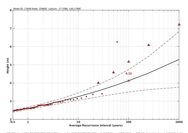
FIGURE 11. AVERAGE RECURRENCE INTERVAL (ARI) CURVE DERIVED FROM THE SCHISM MODEL FOR A SITE NEAR KARUMBA IN THE GULF OF CARPENTERIA. THE HEIGHT OF SEA LEVEL (Y-AXIS) IS SHOWN RELATIVE TO GIVEN ARI IN YEARS (X-AXIS). THE THE BLACK DOTS REPRESENT MODEL SEA LEVEL ANNUAL MAXIMUMS AND THE RED TRIANGLES INDICATE ARI VALUES CONTAINED IN THE SYNTHETIC TROPICAL SYCLONE HAIGH ET AL. 2014 DATASET WHERE THEY EXCEED THE BLACK CURVE
