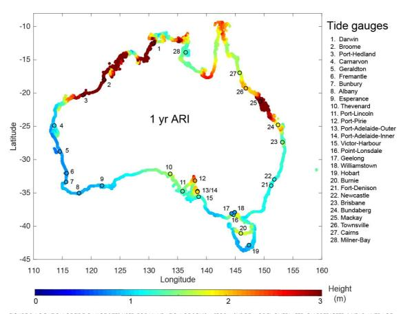
FIGURE 3. LOCATION OF TIDE GAUGE SITES USED FOR VALIDATION OF SCHISM STORM SURGE MODEL OVERLATED ON PREDICTED 1 YEAR AVERAGE RECURRENCE INTERVAL AS AN INDICATOR FOR TIDAL RANGE AROUND AUSTRALIA.
