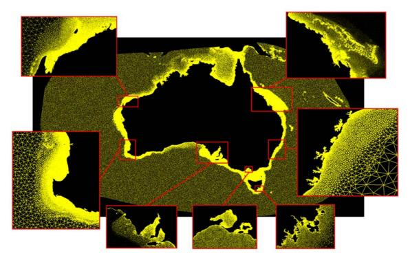
FIGURE 1. SCHISM NUMERICAL MODEL DOMAIN WITH SUBSETS ILLUSTRATING HIGHER RESOLUTION AT THE COAST. SPATIAL RESOLUTION AT THE COAST RANGED FROM 100 TO 800 METRES AND DECREASED OFFSHORE.
