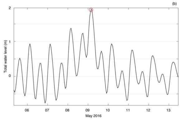
FIGURE 7. PREDICTED TOTAL WATER LEVELS AT THEVENARD, SA FOR ALL OF 2016 (A) AND FOR THE HIGHEST RECORDED SEA LEVEL EVENT ON 9 MAY 2016 (B), CAUSED BY LARGE STORM SURGE COINCIDING WITH HIGH SPRING TIDES. THEVENARD EXPERIENCED A HIGH FREQUENCY OF STORM SURGES DURING 2016 THAT WERE SUCCESSFULLY REPRODUCED BY THE HYDRODYNAMIC MODEL
