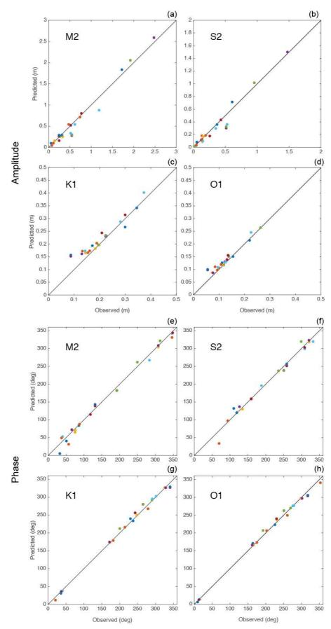
FIGURE 4. OBSERVED VS. PREDICTED AMPLITUDE (A-D) AND PHASE (E-F) OF THE FOUR MAIN TIDAL CONSTITUENTS AT 28 TIDE GAUGE SITES OBTAINED THOUGH HARMONIC ANALYSIS OF PREDICTED AND OBSERVED TOTAL WATER LEVELS.
