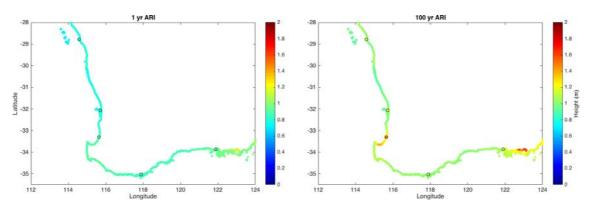
FIGURE 14. ESTIMATES OF 1YEAR AND 100 YEAR TOTAL SEA LEVEL ARI FOR SW WESTERN AUSTRALIA DERIVED FROM THE NUMERICAL MODEL (COLOURED DOTS) AND TIDE GAUGE OBSERVATIONS (BLACK BORDERED CIRCLES).
