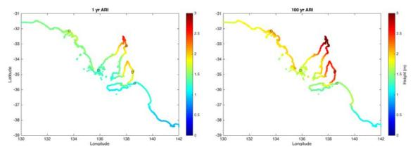
FIGURE 15. ESTIMATES OF 1YEAR AND 100 YEAR TOTAL SEA LEVEL ARI FOR SOUTH AUSTRALIA DERIVED FROM THE NUMERICAL MODEL (COLOURED DOTS) AND TIDE GAUGE OBSERVATIONS (BLACK BORDERED CIRCLES).
