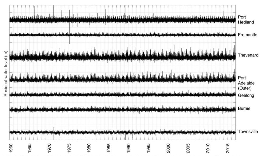
FIGURE 6. PREDICTED NON-TIDAL RESIDUAL SEA LEVELS AT A SELECTION OF SITES, STARTING IN PORT HEDLAND, WA AND MOVING ANTICLOCKWISE AROUND THE COAST. DATA ARE PLOTED WITH AN ARBITRARY OFFSET AND TICK MARKS AT 1 M INTERVALS ON THE Y-AXIS.
