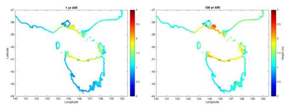
FIGURE 16. ESTIMATES OF 1YEAR AND 100 YEAR TOTAL SEA LEVEL ARI FOR SOUTH EAST AUSTRALIA DERIVED FROM THE NUMERICAL MODEL (COLOURED DOTS) AND TIDE GAUGE OBSERVATIONS (BLACK BORDERED CIRCLES).
