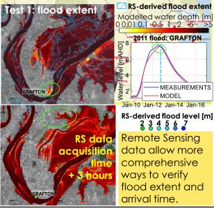
Use of **Remote Sensing-derived** river width, flood extent, and level enables **more accurate modelling of floodplain inundation dynamics**.
