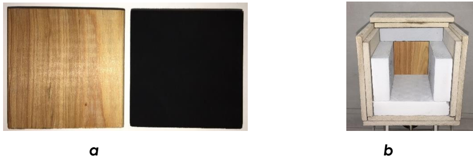
Figure 2 – a) Original (left) and blackened (right) sample; b) sample holder to block convective cooling
