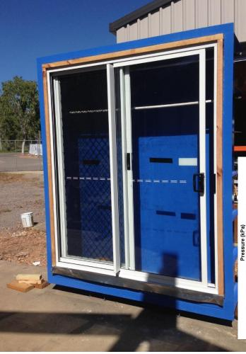
Investigate WDRWI from applying a windward wall fluctuating pressure as opposed to static pressure from the standard
