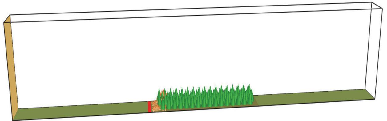
Figure 1. Graphical representation of surface fire-crown interaction simulation
