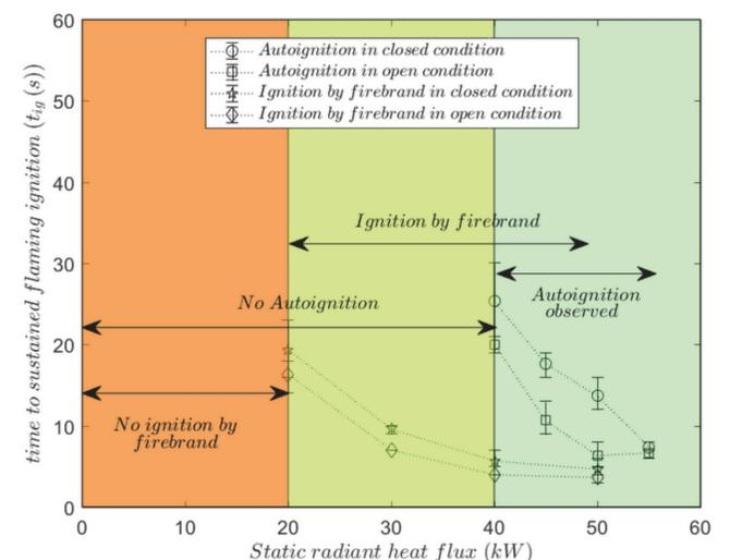
Fig.2: Time to sustained flaming ignition for eucalyptus leaves at different heat flux
