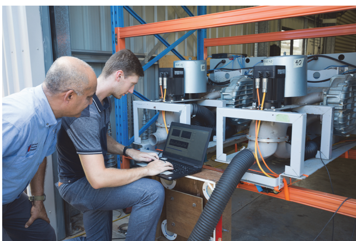
Testing using Pressure Loading Actuators
