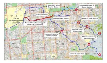
FIGURE 2. LOCATION OF FLOOD-CONTROL DAMS FOR OPTIONS B1 AND B2 (SOURCE: BHKCP, 2016)
