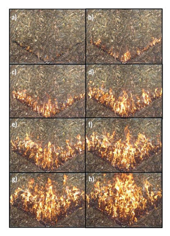
**Figure 3:** a-h) Series of rectified and corrected images taken from the planar video from one replication of the no-wind experiment using an 800 mm ignition line and 60° incidence angle. The images show the progression of the fire every 5 seconds after ignition (panel a). The flame front was defined as the leading edge of combustion at the fuel level as determined from multiple viewing angles, not to be confused with the presence of flame. The image was taken from Sullivan et al (2017).
