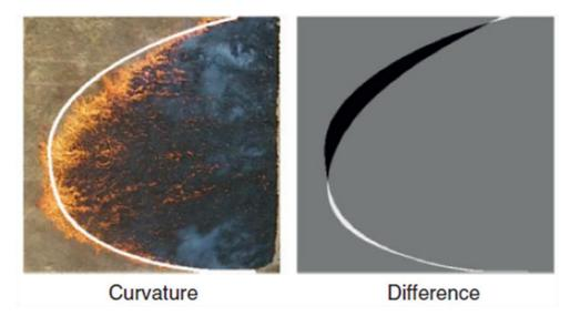
**Figure 6:** Left: Image of experimental grassfire 25 seconds after ignition. The white line is the model prediction. Right: difference between stencils from experimental and simulated perimeters with curvature effects. Figure taken from HIIton et al. (2016).
