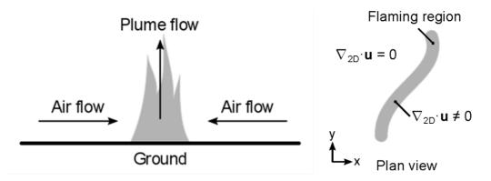
**Figure 7:** Left: Schematic view of the indraft into a fire plume. Right: Schematic view of a fire line as a sink for the horizontal indraft into the fire's plume.
