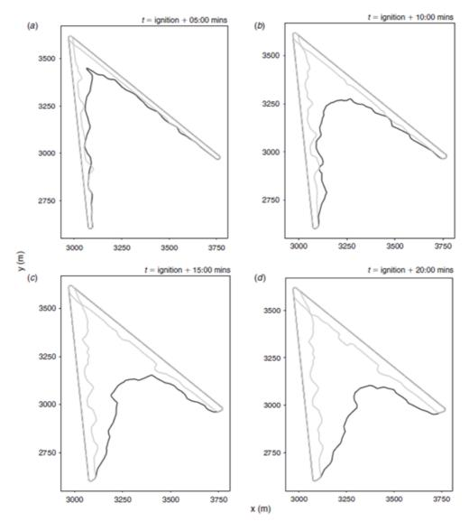
**Figure 4**: Composite plot of three model runs of the 45° configuration, shown (a) 5; (b) 10; (c) 15; and (d) 20 min after ignition. The grey lines show the evolution of the front when only one arm of the V is ignited; together, they show how the front would evolve without interaction between the two fire lines. The black line shows the evolution when both arms are ignited simultaneously. Figure taken from Thomas et al. (2017).
