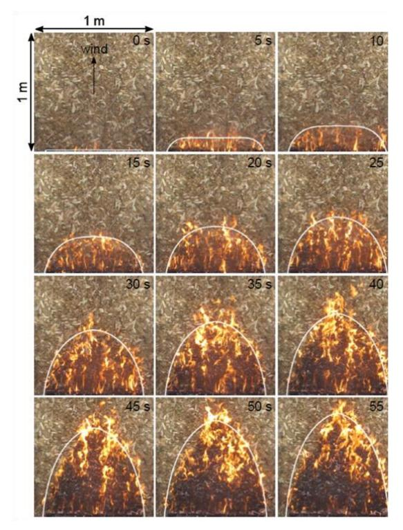
**Figure 9:** Comparison of laboratory experimental line fire to a basic propagation model incorporating a pyrogenic potential term, where the white line is the simulated fire perimeter, at 5 s intervals. Wind speed is 1 m/s in the direction indicated by the arrow in the first image.
