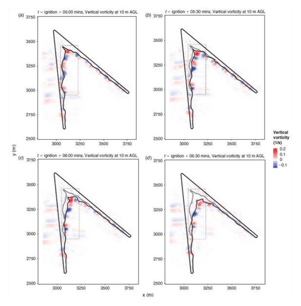
**Figure 5:** Advection and merging of counter-rotating vortex pairs. The time sequence shows the fire line location and vertical vorticity for one 45° ensemble member at 30s intervals, beginning 5 min after ignition. The (stationary) grey line shows the location of the fire line at the initial time of the sequence. Figure taken from Thomas et al. (2017).
