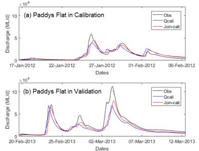
FIGURE 2 STREAMFLOW PREDICTION AT "UNGAUGED" LOCATIONS OF PADDYS FLAT SHOWING ONE FLOOD EVENT IN THE CALIBRATION PERIOD AND ANOTHER IN THE VALIDATION PERIOD.
