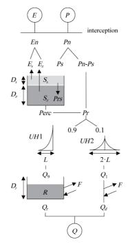
FIGURE 1 THE STRUCTURE OF THE GRKAL MODEL (FRANCOIS ET AL., 2003).
