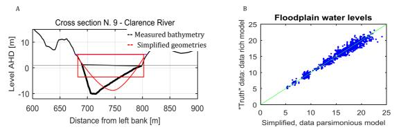
FIGURE 4A - CLARENCE RIVER, EXAMPLE OF CROSS SECTION. BLACK: FIELD DATA; MAGENTA: BANKFULL LEVEL; RED: RECTANGULAR SIMPLIFIED GEOMETRY AND EXPONENTIAL SIMPLIFIED GEOMETRY. FIGURE 4B - COMPARISON OF THE RESULTS OF DATA RICH MODEL WITH THE RESULTS OF THE SIMPLIFIED MODEL
