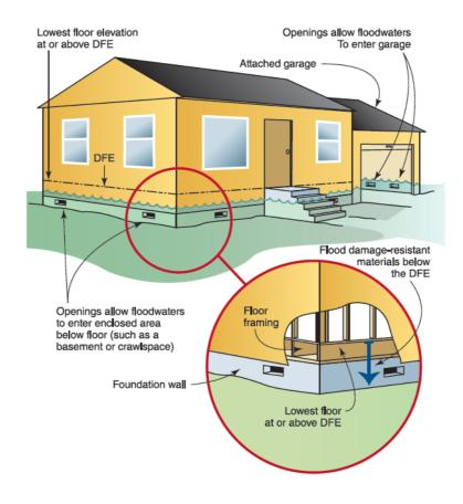
Figure 8. Techniques for wet floodproofing (FEMA, 2000)
