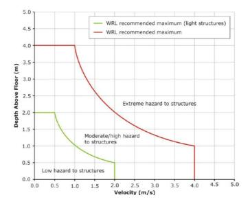
Figure 3. Thresholds for building stability in floods (Smith et al. 2014; McLuckie et al. 2014)
