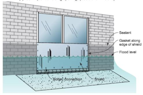
Figure 7. Techniques for dry floodproofing (FEMA, 2000)
