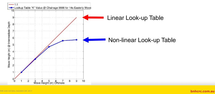
Simulating waves nearshore (SWAN) model coastal wave transformation simulations.
