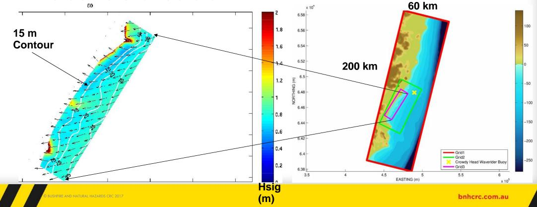
Simulating waves nearshore (SWAN) model coastal wave transformation simulations.
