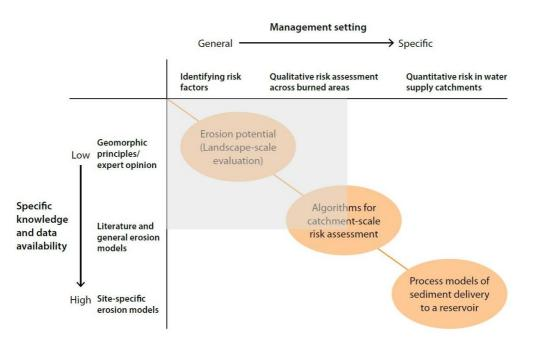
FIGURE 2 - THE TYPES OF MODELS FOR RISK ASSESSMENTS VARY DEPENDING ON THE MANAGEMENT SETTING (TOP AXIS) AND THE SCIENTIFIC KNOWLEDGE (LEFT AXIS) OF THE UNDERLYING HYDRO-GEOLOGICAL PROCESSES. THIS DIAGRAM ILLUSTRATES HOW SCIENCE GAINED FROM ONE SPECIFIC SITE COULD BE TRANSLATED GENERALLY FOR APPLICATION IN DIFFERENT CONTEXTS. THE SHADED AREA REPRESENTS THE REGION OF THE SCIENCE-MANAGEMENT SPACE THAT WAS TARGETED IN THE FIRST PHASE OF UTILISATION.
