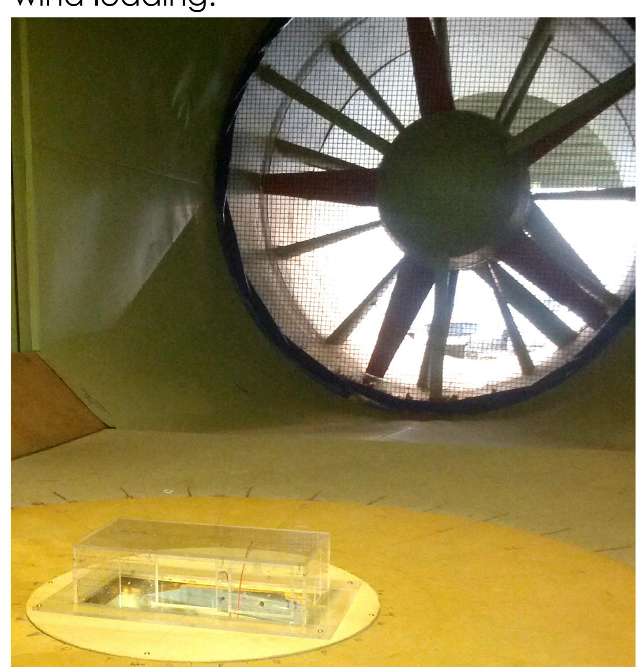
Wind Tunnel Set-up of Scale Model
