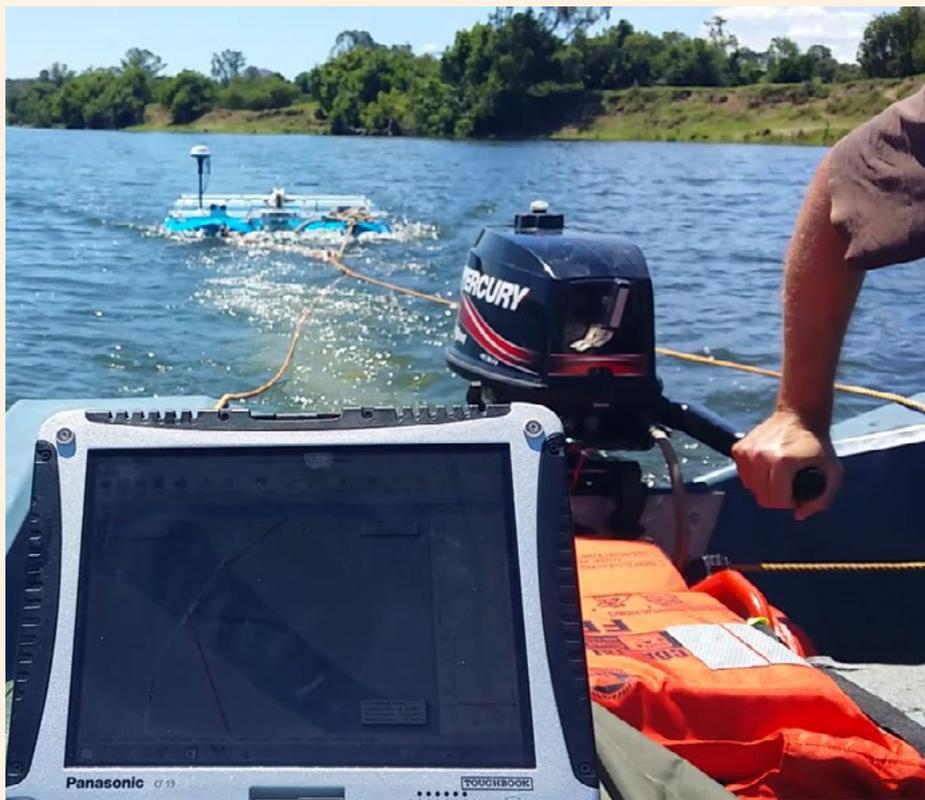
▲ **Above:** THE RESEARCH TEAM USES A RIVERSURVEYOR ACOUSTIC DOPPLER PROFILER TO MEASURE THE TOPOGRAPHY OF THE CLARENCE RIVER UPSTREAM OF GRAFTON. PHOTO: STEFANIA GRIMALDI
