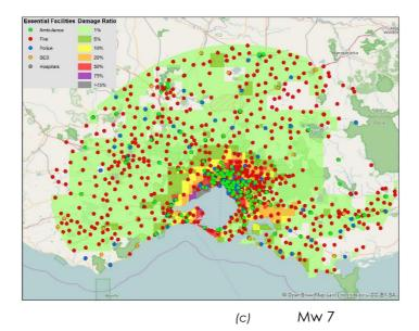
Figure 18: Damage Ratio to essential facilities. Mw = magnitude
