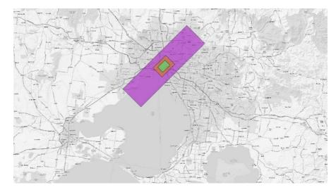
Figure 8: Surface projection of the three considered event fault ruptures. Green: Mw 5.5, Orange: Mw 6 and Purple: Mw 7.
