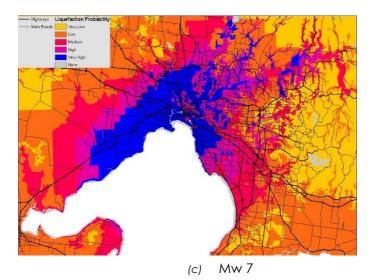
Figure 11: Liquefaction potential map for Melbourne. Hot colours represent areas with higher probability of liquefaction. Mw = magnitude
