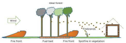
A Above: A SCHEMATIC OF FIRE SPREAD MECHANISM IN THE IDEAL FOREST SHOWING SPOTTING IN VEGETATION AND A MODEL HOUSE.
