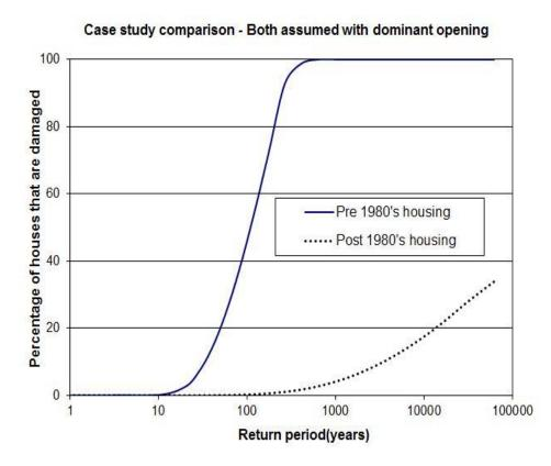
Failure of structural connections in older housing at wind speeds less than design
