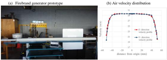
Figure 6: Firebrand generator prototype and air velocity distribution
