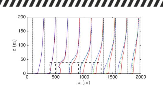
Figure 4: Centreline average streamwise velocity profiles along the 100 m (red solid), 500 m (green dashed), and 900 m (blue dotted) canopies, with fixed LAD profile. The flow develops almost identically within the canopies.
