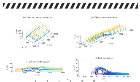
Figure 3: Streamlines within the various flow regimes. The streamlines have been constructed from the time averaged data and coloured by the velocity magnitude. (a) the streamlines around the canopy, (b) the streamlines through the canopy, (c) the edge streamlines, (d) streamlines in the recirculation region showing the presence of a large, but slowly rotating vortex.
