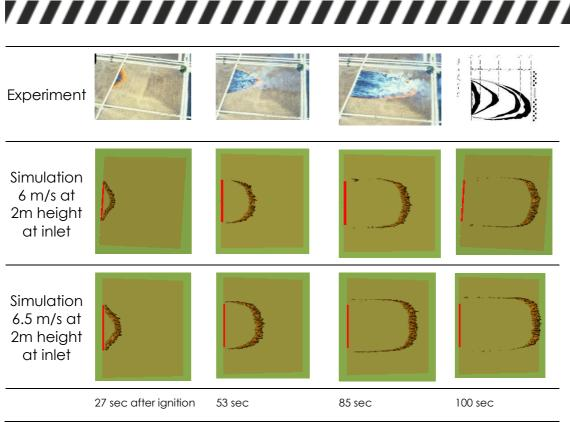
Figure 9: Model validation: fire propagation
