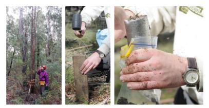
FIGURE 2. FIELD TECHNIQUES; MEASURING TREE HEIGHT (LEFT), INSERTING SOIL CORE (MIDDLE) COLLECTING SOIL FOR MEASUREMENT BULK DENSITY (RIGHT)
