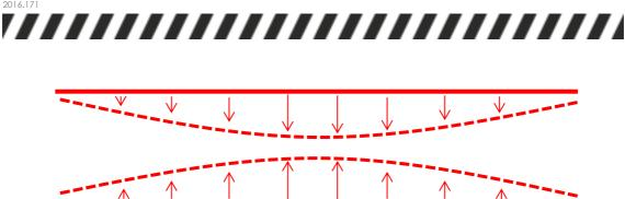
**Figure 3:** Schematic representation of two straight, parallel fire lines (solid lines) burning towards each other. The dashed lines indicate the fire lines at some subsequent time and portray the effect of the dynamic interaction between the two fire lines. The arrows represent the relative rates of spread of different parts of the fire lines.
