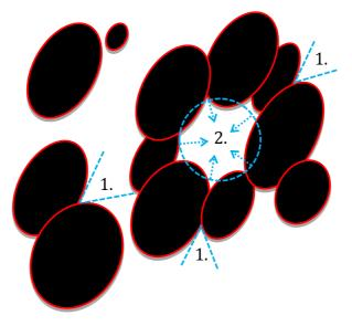
**Figure 1:** Schematic representation of coalescing spot fires. Examples of fire line merging are marked with a 1, while an example of perimeter collapse is marked with a 2. Both phenomena involve changes in topology.
