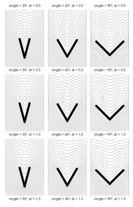
**Figure 2:** Computational simulations of 'V-shaped' fire isochrones for a range of interior angles and strengths of curvature dependence (described by parameter  $\alpha$ ). The other model parameters are fixed:  $\beta = 0.2$  and  $\gamma = 0.3$ .
