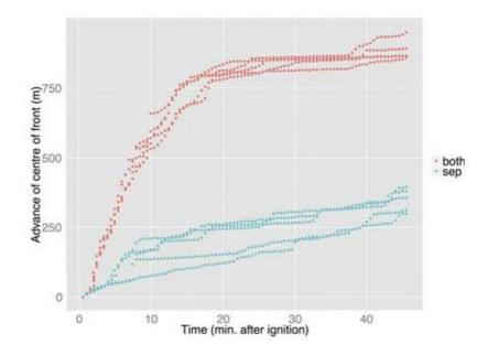
**Figure 5:** Fire front advance over time for a V-shaped fire with fire lines meeting at 30°. The figure shows the results for various ensemble members. Red points represent spread when both arms of the 'V'-configuration are ignited simultaneously. Blue points indicate spread when each arm is ignited individually (representing the decoupled case). Figure adapted from Thomas et al. (2016).
