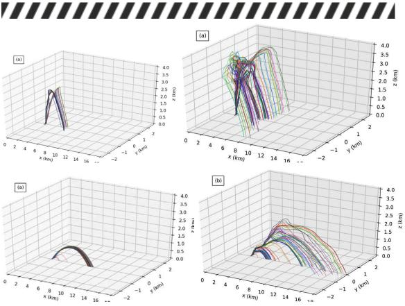
FIGURE 2. TRAJECTORIES OF 100 FIREBRANDS LOFTED BY THE MEAN (LEFT) AND TIME-VARYING (RIGHT) PLUMES UNDER BACKGROUND WIND SPEEDS OF 5 (TOP) AND 15 (BOTTOM) M S–1.
