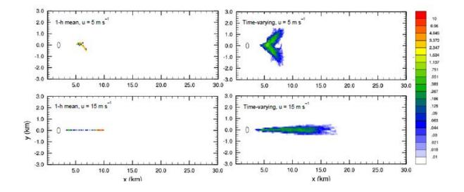
FIGURE 3. SPATIAL DISTRIBUTIONS OF FIREBRAND LANDING POSITION (PERCENT OF PARTICLES LAUNCHED PER KM2) FOR THE MEAN (LEFT) AND TIME-VARYING (RIGHT) PLUMES UNDER BACKGROUND WIND SPEEDS OF 5 (TOP) AND 15 (BOTTOM) M S–1.
