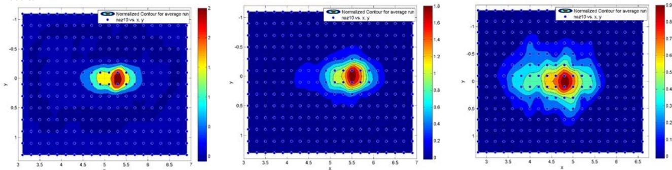
Fig. 1: Normalized distribution of non-burning firebrands after 10 experimental runs for (a) cubical, (b) cylindrical, and (c) square disc
