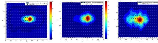
Fig. 1: Normalized distribution of non-burning firebrands after 10 experimental runs for (a) cubical, (b) cylindrical, and (c) square disc
